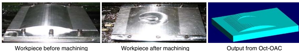
Fig. 26 View of the circular hole milling
